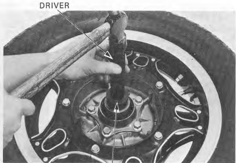
DRIVER ATTACHMENT 42 x 47 mm AND PILOT 15 mm
