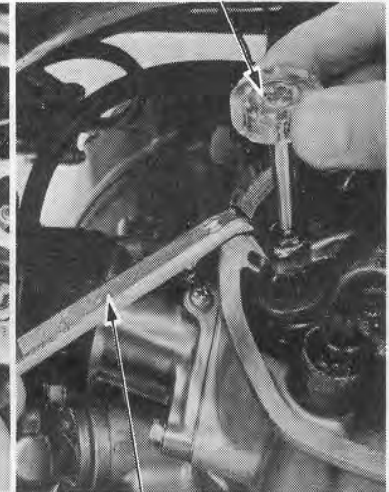
VALVE ADJUSTING WRENCH 10 x 12 mm
